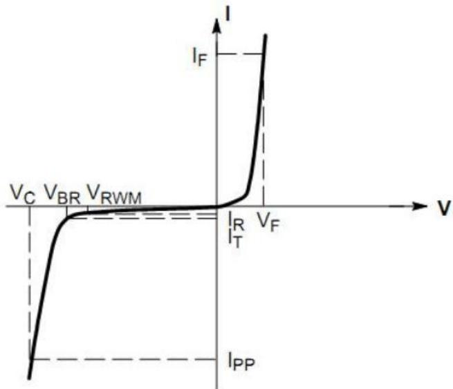
**■Typical Characteristic Curve 典型特性曲线**
