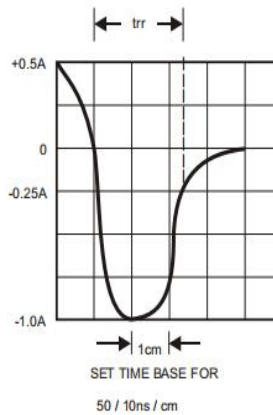
FIG.1- TEST CIRCUIT DIAGRAM AND REVERSE RECOVERY TIME CHARACTERISTIC
