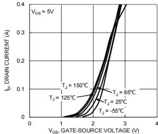
Figure 2: Transfer Characteristics
