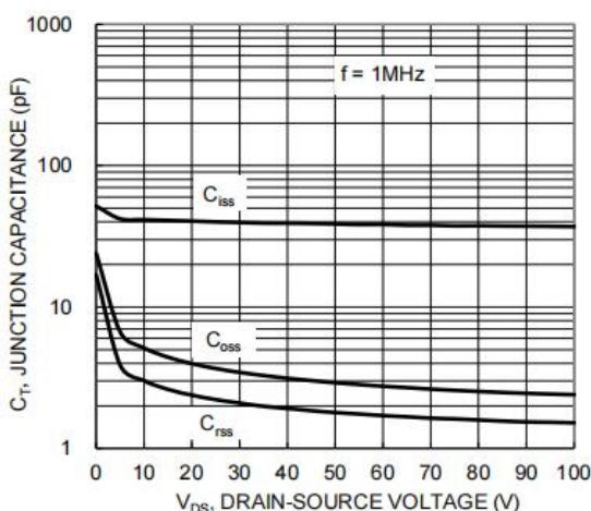
Figure 5: Capacitance Characteristics
