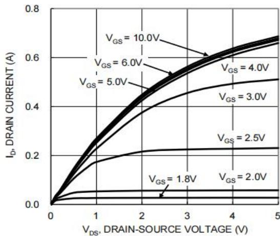
Figure 1: Output Characteristics
