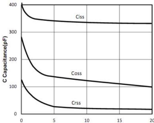
**V<sub>DS</sub> Drain-Source Voltage (V)**
