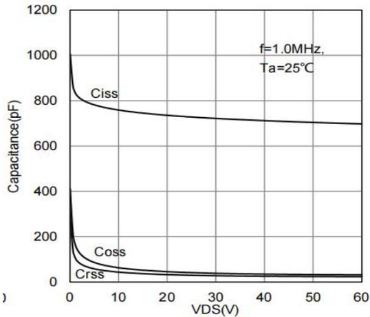
Figure 5: Capacitance Characteristics
