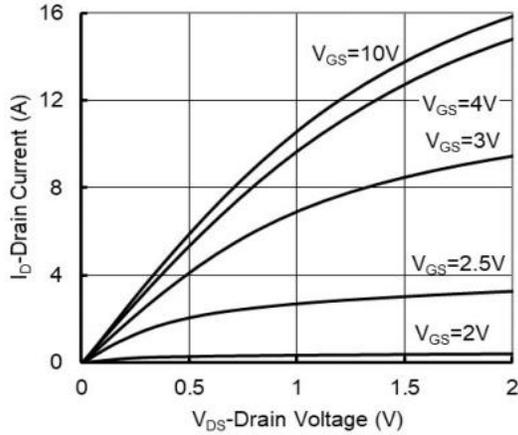
Figure 1: Output Characteristics
