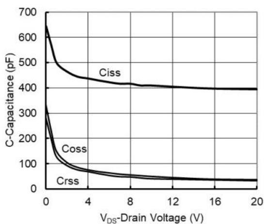
Figure 5: Capacitance Characteristics
