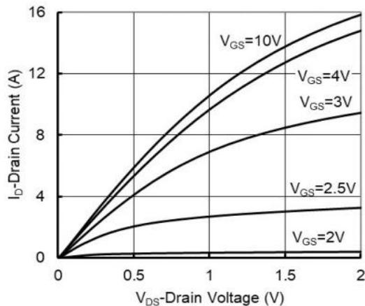
Figure 1: Output Characteristics
