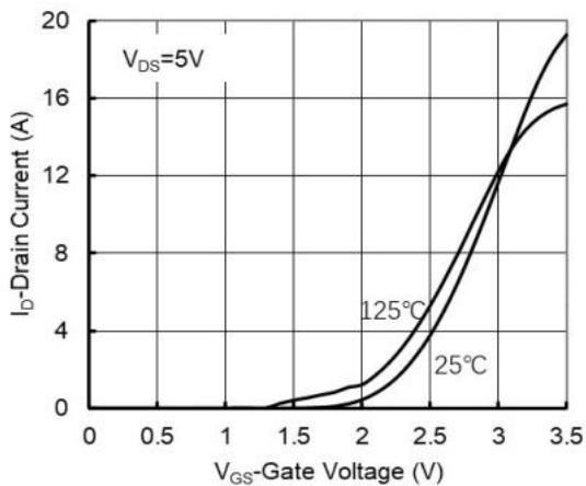
Figure 2: Transfer Characteristics
