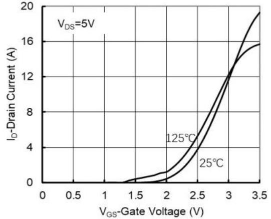
Figure 2: Transfer Characteristics
