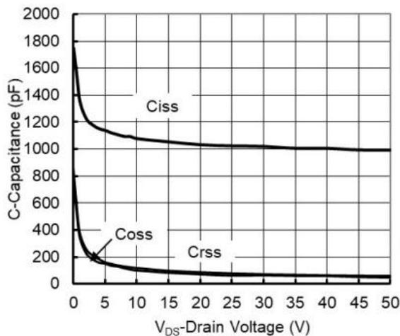
Figure 5: Capacitance Characteristics
