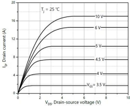
Figure 1: Output Characteristics
