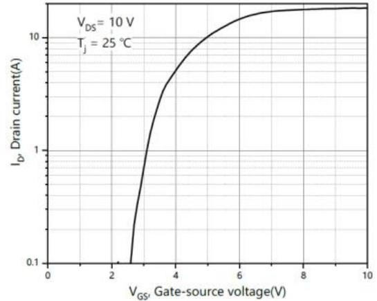
Figure 2: Transfer Characteristics
