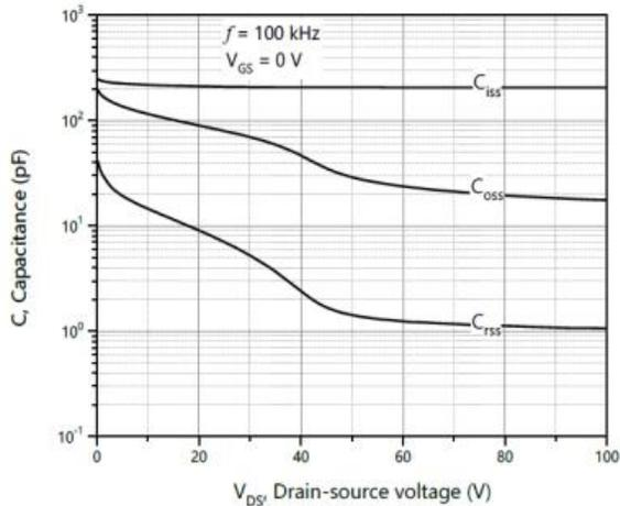
Figure 5: Capacitance Characteristics
